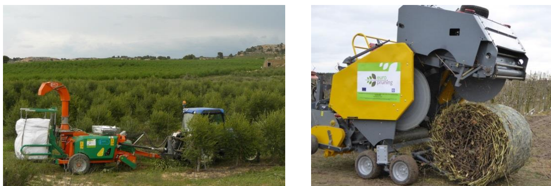
Figure 22: Two examples of innovative solutions for harvesting wood from agricultural prunings developed through the EuroPruning project: ONG-SNC chipper PC50 capable of discharging on big-bags, trailer circulating in parallel, or on a built-in container with capacity to tilt and discharge (left); Round baler PIMR PC50 (right).
